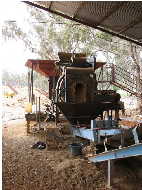
Figure 3 View of the GeoBrick batch mixing machinery at their operations in Bealiba.
